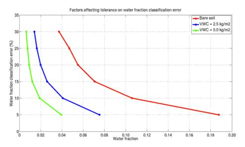
Figure 13. For a given soil moisture retrieval RMSE ( $0.005~\rm cm^3/cm^3$  in this case), more accurate estimation of the water fraction is needed for  $T_B$  observations that contain a larger water fraction and/or a larger vegetation water content.
