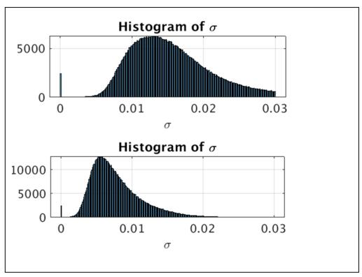
Figure 17. Histograms of  $\sigma$  , standard deviation of the Nyquist frequency of DCA  $\tau$  before (top) and after (bottom) regularization.
