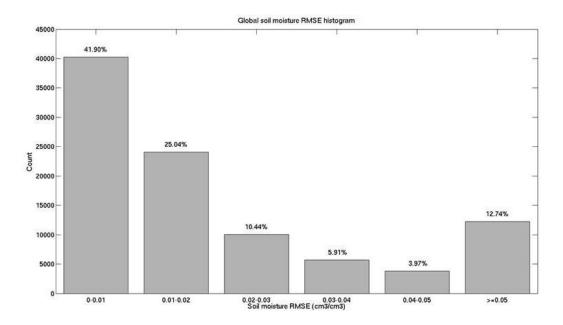
Figure 22b. Histogram of global soil moisture retrieval error based on simulation shown in (a). Approximately 83% of the area in the SMAP land mask has a soil moisture retrieval error  $\leq 0.04 \text{ cm}^3/\text{cm}^3$ .
