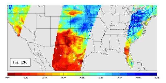
Figure 12. Simulation of L3\_SM\_P retrieved soil moisture in cm<sup>3</sup>/cm<sup>3</sup>. This example is based on the single channel algorithm operating on H-polarized T<sub>B</sub> observations simulated using geophysical data from a land surface model.
