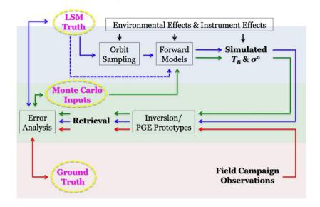
Figure 21. The various simulation modules and input data sources for the SMAP Algorithm Development Testbed.
