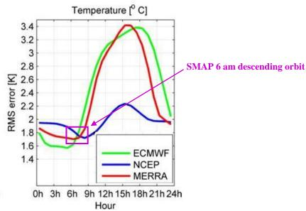
Figure 24. Accuracy of NWP forecast surface soil temperature compared against in situ temperatures for the Oklahoma Mesonet for 2004 and 2009.
