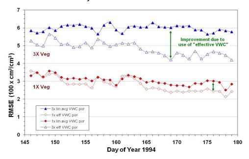
Figure 15. Improvement in simulated Hydros soil moisture retrieval error using a simple effective VWC correction with the SCA algorithm for existing vegetation (1X) and for artificially increased simulated vegetation amounts (3X) [31].
