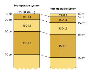
In the upgraded GEOS system, *Tsurf* is a temperature prognostic that is formed based on bare soil, vegetation, and snowpack temperatures in proportion to their prevalence across the pixel area. This temperature is a flux temperature which is used in the gradient-driven exchanges of heat between the surface and the atmospheric boundary layer. *TSOIL*1 and *TSOIL*2 are consistently soil media temperature prognostic variables that are characterized by these extensive attributes:
