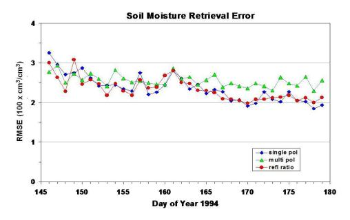
Figure 29. Performance comparison among three candidate retrieval algorithms for the *Hydros* mission based on an OSSE over the Arkansas-Red River basin [7].
