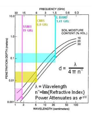
Figure 4. L-band  $T_B$  observations are sensitive to emission from deeper in the soil than at higher frequencies [adapted from 23]. Soil moisture curves are given for 10, 20, and 30% (or in absolute units, 100 x cm<sup>3</sup>/cm<sup>3</sup>).
