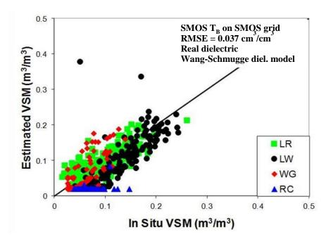
Figure 20. Comparison of estimated soil moisture using SMOS-simulated SMAP  $T_B$  with in situ observations over USDA ARS watershed sites for ascending orbits (6 AM overpass time) for January 2010-May 2013. One of the two outliers is due to the likely presence of wet snow not predicted by ECMWF; the other outlier is due to an unpredicted active rain event.
