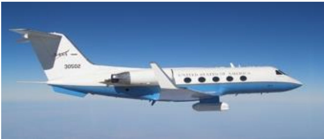
Figure C-9-2. The UAVSAR instrument in the belly pod of NASA Gulfstream III aircraft.
