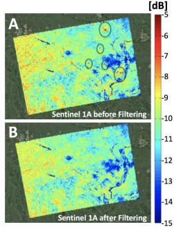
**Figure 9**: Sentinel-1A  $\sigma_{vv}$  granule from Southern Iowa on May 05, 2018. (A)  $\sigma_{vv}$  unprocessed data; and (B)  $\sigma_{vv}$  data after calibration, noise subtraction, terrain correction (using SRTM DEM), filtering, and aggregation to 1 km.
