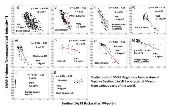
**Figure 3**: Scatter plots between the SMAP L-band radiometer  $T_{B_p}(C)$  and spatially-averaged Sentinel C-band radar data  $\sigma_{nn}(C)$  from various regions of the world.
