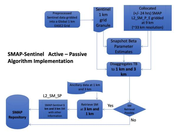
**Figure 8**: Process flow scheme of the SMAP-Sentinel-1A/1B Active-Passive (L2\_SM\_SP) algorithm in the JPL SDS.
