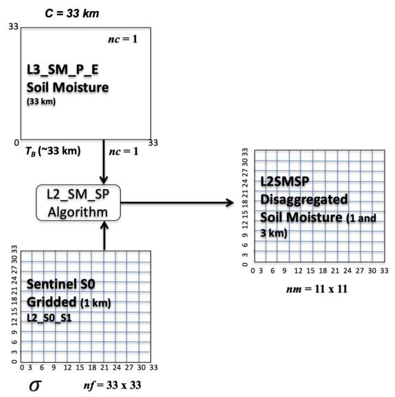
**Figure 2**: Grid definition of radiometer, radar, and merge product where nf and nm are the number of area pixels of radar and merged product, respectively, within one radiometer area pixel nc.
