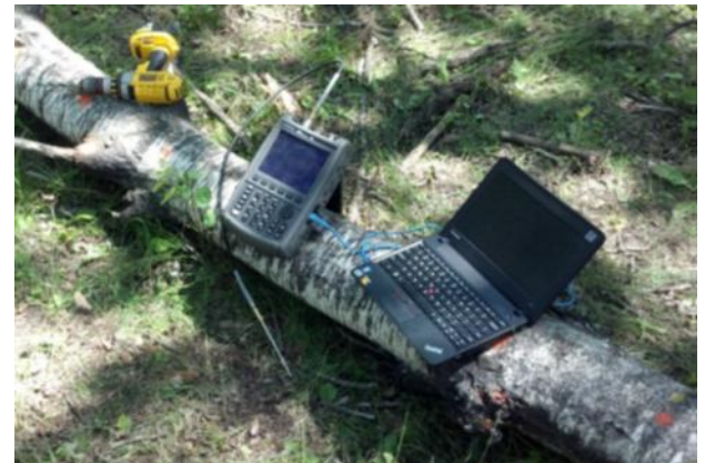
Dielectric measurement using an Agilent field portable network analyzer (FieldFox N9923A)
