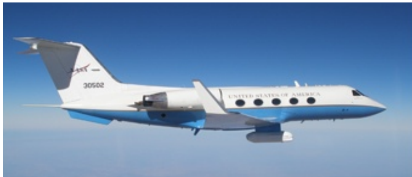
Figure C-2. The UAVSAR instrument in the belly pod of NASA Gulfstream III aircraft.
