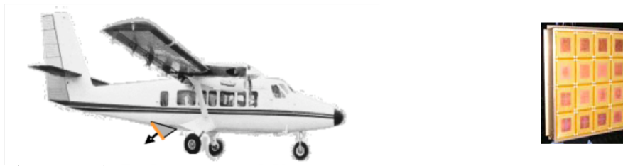
Figure C-1. Twin Otter (on the left-hand side) and light-weight relative small-size microstrip antenna (on the right-hand side)
