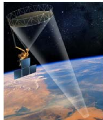
Figure 1. SMAP observatory with spinning 6m deployable mesh reflector antenna. The active radar and passive radiometer share a common L-band feed horn.
