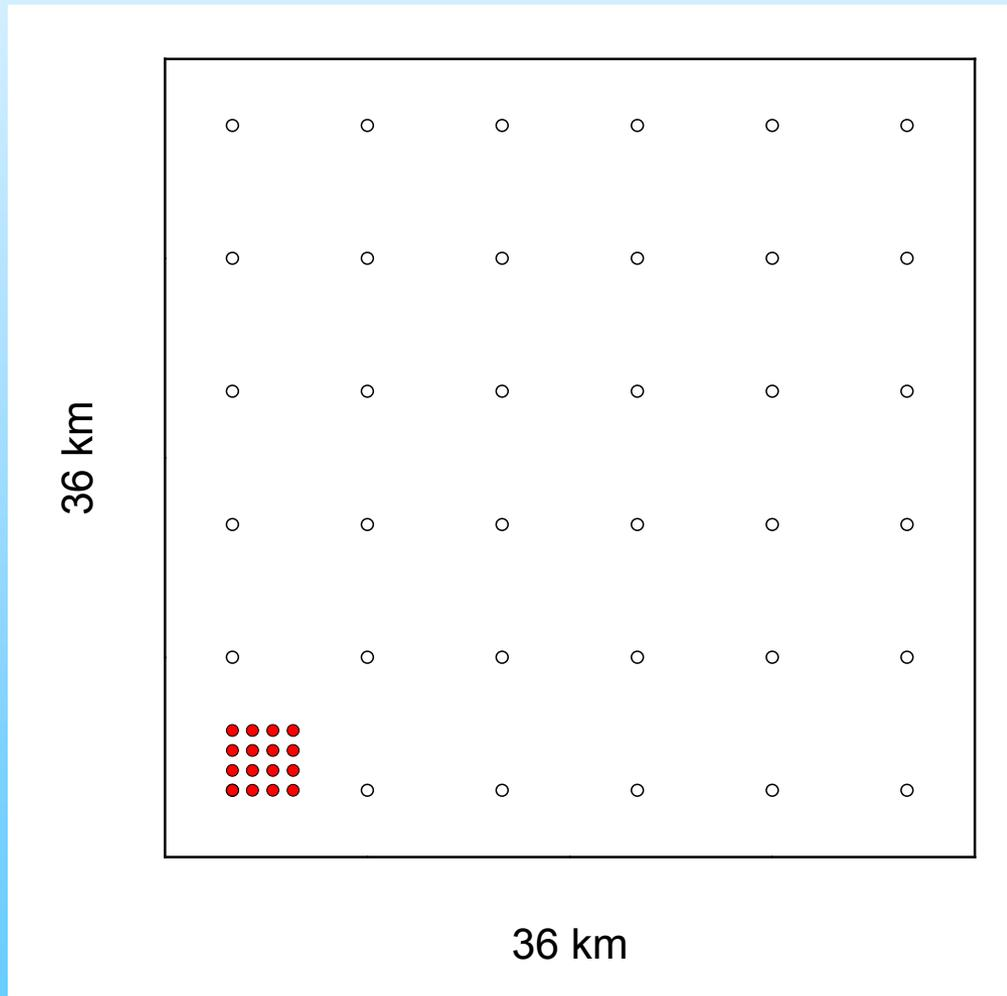
Need 30+ probes to capture soil moisture variations and obtain representative soil moisture fields within the passive pixel area.
