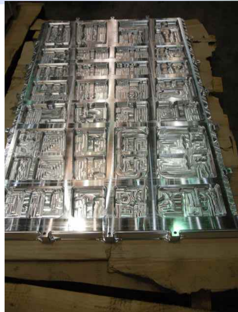
Spacecraft -Y Panel (Radar Panel) in rough machining
