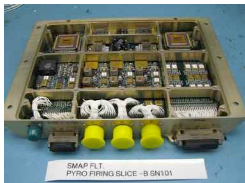
Pyro Firing Slices are Assembled and Tested
