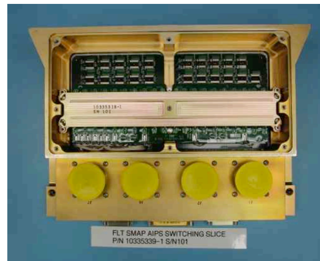
Flight Solar Array Interface & Switching Slice
