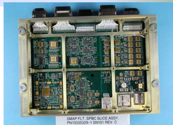
Flight Spacecraft Power Bus Controller Slice
