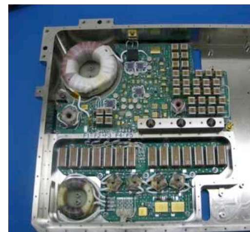
High Power Amplifier is in Assembly
