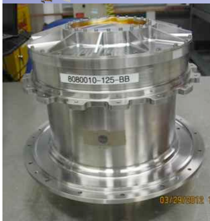
Brassboard Bearing & Power Transfer Assembly (BAPTA)
