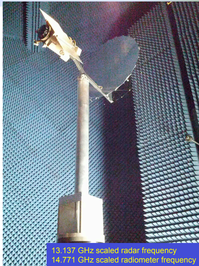
SMAP Scale Model Observatory being Tested in JPL's Cylindrical Near Field Range (Mesa 40' chamber)
