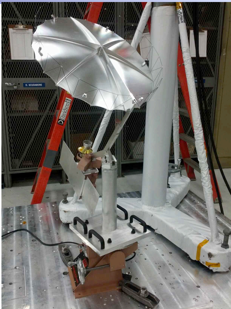
SMAP Scale Model Observatory (10.45 to 1 scale)
