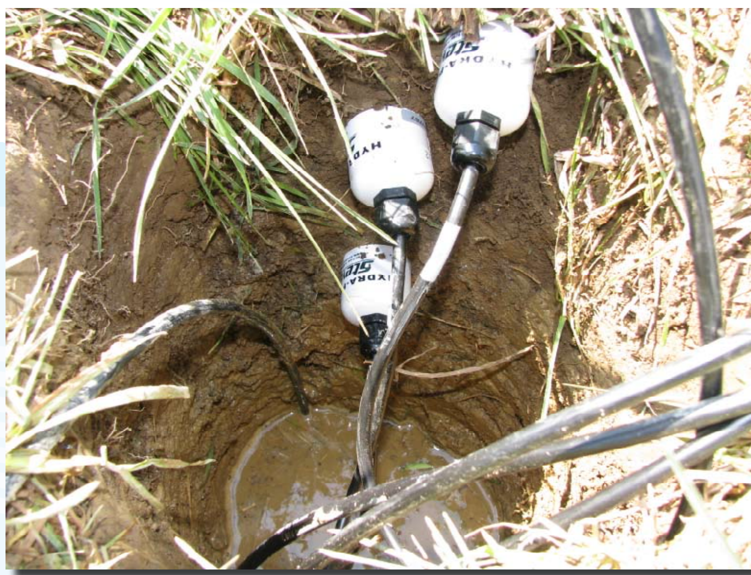
Initial installation of soil probes at Crossville, Tennessee, April 2009.
