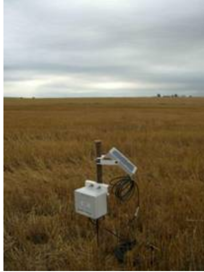
Figure 7. Example of temporary stations installed with a solar panel and CR206 logger. A Stevens Hydra Probe and a CS655 reflectometer are installed at a depth of 5 cm to mimic the long term in situ station.
