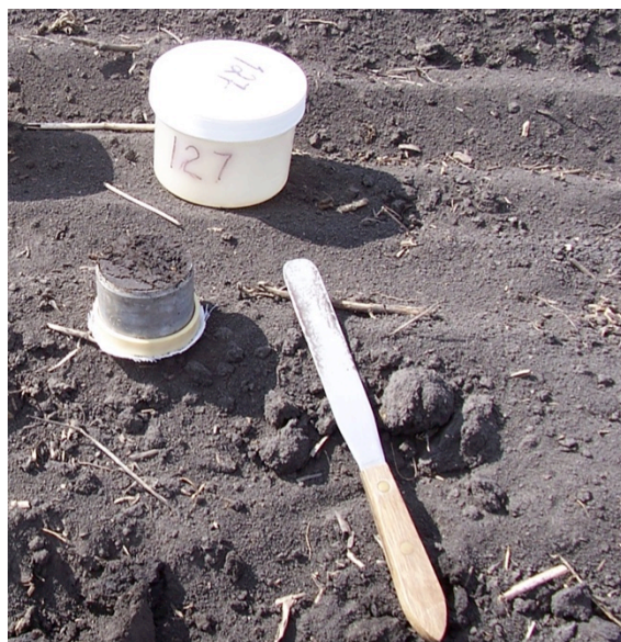
Figure 26. A sample that has been trimmed to size and now ready to be transferred to the sample container.
