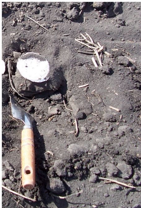
Figure 25. Loosening a sample ring to remove the sample from the soil.
