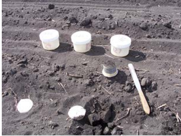
Figure 31. A sample that has been trimmed to size and now ready to be transferred to the sample container
