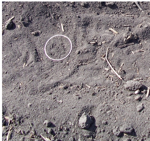
Figure 24. Aluminum sampling ring fully inserted. Three POGO samples can be taken surrounding the ring approximately 10 cm away.
