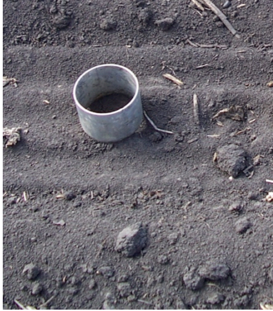
Figure 23. Aluminum sampling ring ready to be inserted at a volumetric soil moisture calibration sample location.
