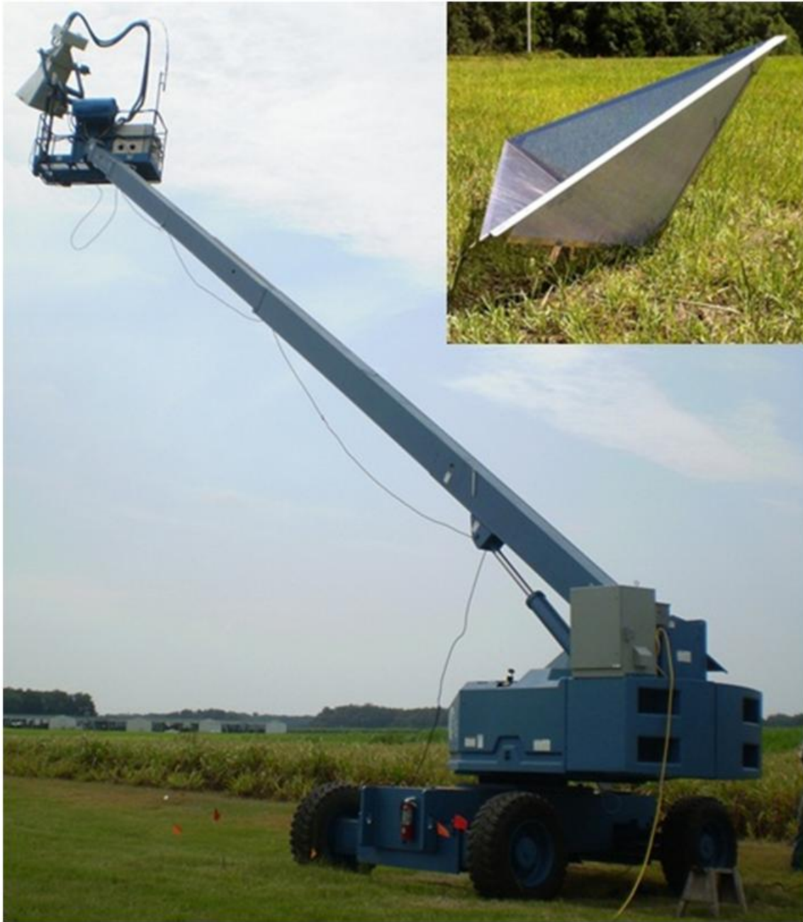
Figure 15: UF-LARS mounted on the 25 m Genie platform. (Inset) Trihedral calibration target made of aluminum with an aperture length of 1.28 m. Credits: Karthik Nagarajan, University of Florida
