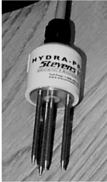
Figure 36: The Hydra probe used at the tower locations.
