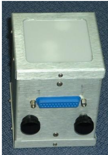
Figure 38: CROPSCAN Multispectral Radiometer (MSR). (Size is 8 X 8 X 10 cm).
