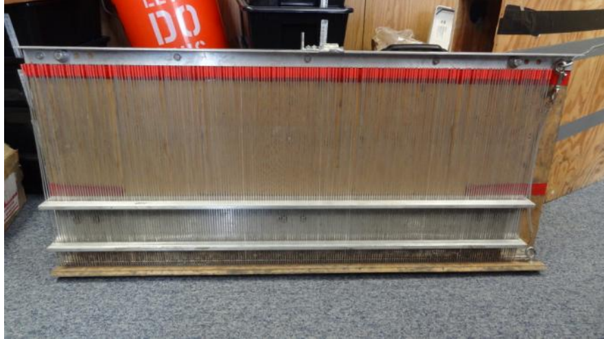
Figure 34: Pin board to be used for surface roughness measurements.
