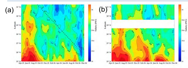
Hovmöller diagrams using SMAP-derived SSS of the latitudinal variation at two ((a) 120W and (b) 118W) longitudes. The dashed line shows the approximate propagation of the freshening from north to south.
