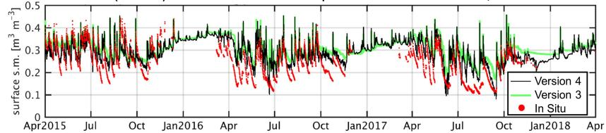
**Finding**: The Level-4 (L4) algorithm assimilates SMAP brightness temperature observations into the Catchment land surface model. Model bias adversely impacts L4 estimates. The model bias was caused in part by excessive coupling between the surface and deeper-layer soil moisture. The upward recharge of surface soil moisture from deeper layers was reduced in the Version-4 system, resulting in model and L4 estimates with reduced bias and improved dynamic range.
