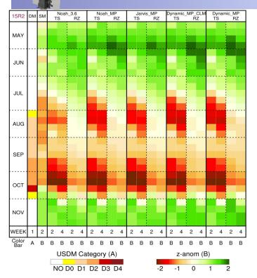
Drought evolution across the south-central U.S. in 2015. The USDM analysis is shown in column 1 followed by anomalies of SMAP in column 2. Anomalies (based on 1979-2017) of top soil (TS) and root zone (RZ) soil moisture from the Noah 3.6, Noah-MP, Jarvis-MP, Dynamic-MP-CLM, and Dynamic MP simulations are shown in subsequent columns.
