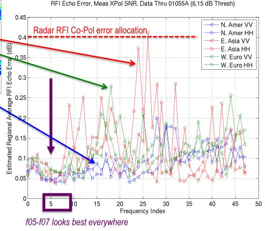
RFI environment is manageable with one transmit frequency globally
