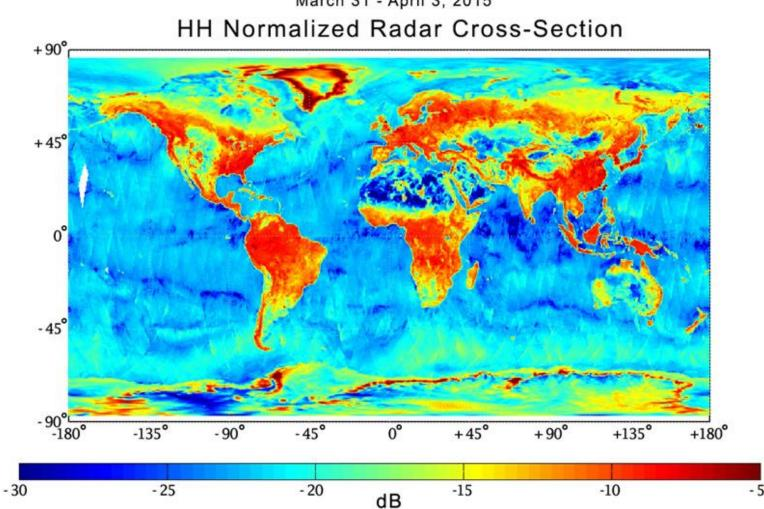
Sigma-0 HH from low-res radar L1B; 3-day collection from timing test
