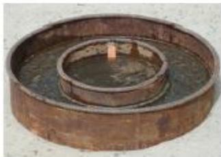
a) Twin Ring Infiltrometer
