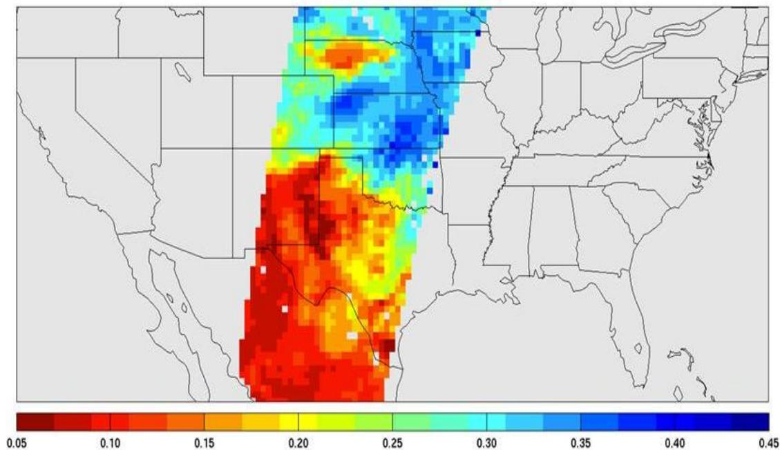
**Figure 11. Example of SMAP retrieved soil moisture in  $\text{cm}^3/\text{cm}^3$ . The half-orbit swath pattern is simulated using the orbital sampling module on the SMAP Algorithm Development Testbed.**
