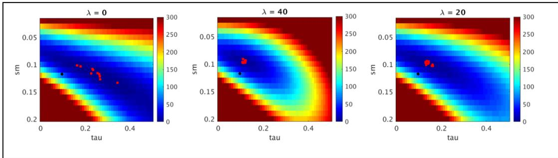
**Figure 16. Image of the cost function  $F$  for different values of lambda. From left to right:  $\lambda = 0$ ,  $\lambda = 40$  and  $\lambda = 20$ . The black dot represents the initial value and the red dots are the solution for different realizations of the perturbed brightness temperatures.**
