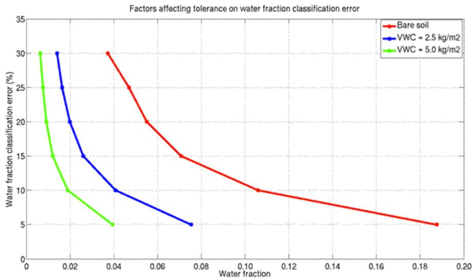
**Figure 13. For a given soil moisture retrieval RMSE ( $0.005 \text{ cm}^3/\text{cm}^3$  in this case), more accurate estimation of the water fraction is needed for  $T_B$  observations that contain a larger water fraction and/or a larger vegetation water content.**
