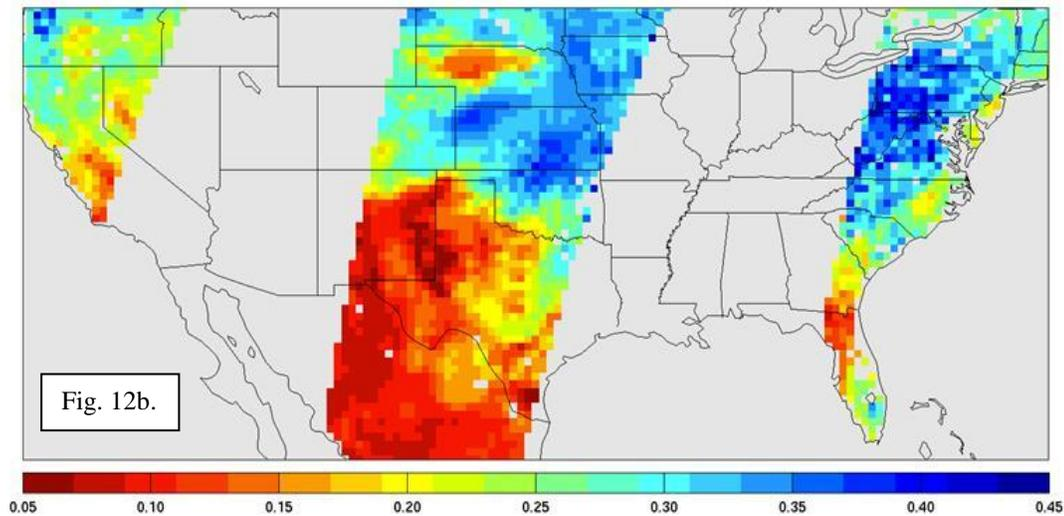
**Figure 12. Simulation of L3\_SM\_P retrieved soil moisture in  $\text{cm}^3/\text{cm}^3$ . This example is based on the single channel algorithm operating on H-polarized  $T_B$  observations simulated using geophysical data from a land surface model.**
