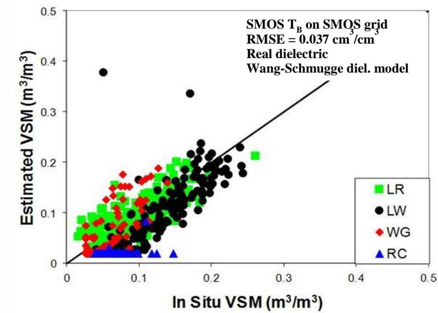
Figure 20. Comparison of estimated soil moisture using SMOS-simulated SMAP T<sub>B</sub> with *in situ* observations over USDA ARS watershed sites for ascending orbits (6 AM overpass time) for January 2010-May 2013. One of the two outliers is due to the likely presence of wet snow not predicted by ECMWF; the other outlier is due to an unpredicted active rain event.
