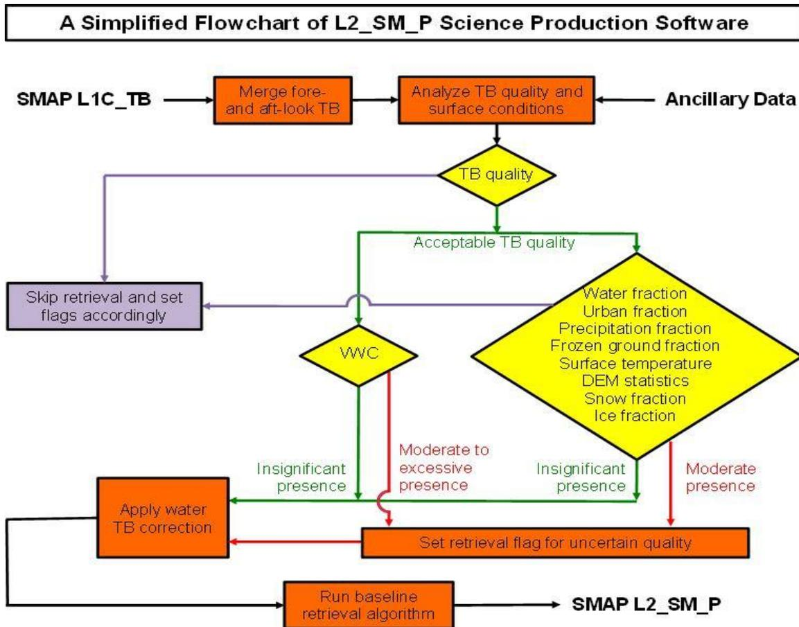
**Figure 10. Conceptual flow of L2\_SM\_P process from input of T<sub>B</sub> to output of retrieved soil moisture.**
