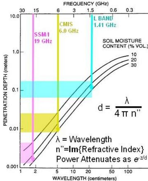
**Figure 4.** L-band  $T_B$  observations are sensitive to emission from deeper in the soil than at higher frequencies [adapted from 23]. Soil moisture curves are given for 10, 20, and 30% (or in absolute units,  $100 \times \text{cm}^3/\text{cm}^3$ ).
