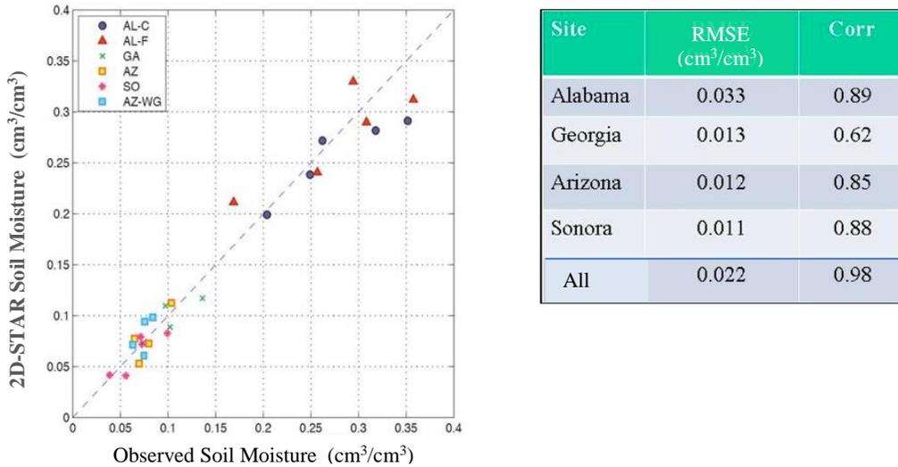
**Figure 14. Soil moisture retrieval error based on L-band H-polarized  $T_B$  airborne observations. The vegetation parameter  $b$  and roughness parameter  $h$  are optimized using ground measurements of soil moisture from the SMEX03 and SMEX04 field campaigns [30]; also D. Ryu, personal communication]. The canopy and soil temperatures are assumed to be equal (i.e.,  $T_c = T_s = T_{eff}$ ) under the hydraulic equilibrium assumption.**
