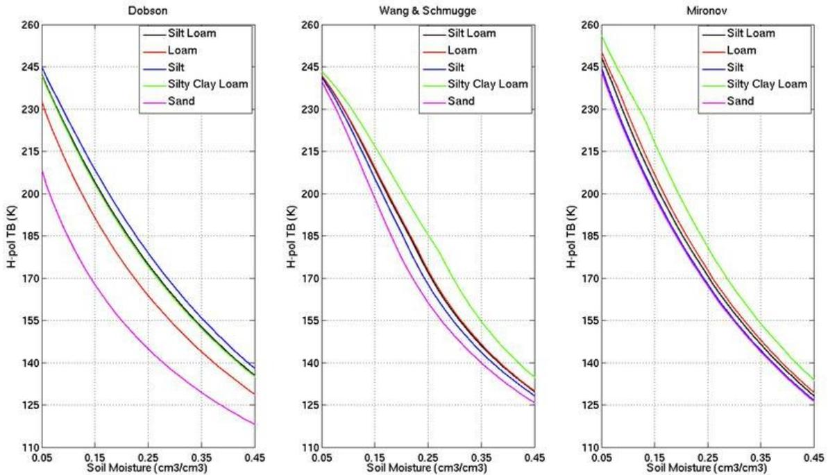
**Figure 5. Bare soil  $T_B$  as computed by different soil dielectric models. The selected soil types correspond to the top five most dominant soil texture classes, together accounting for over 80% of the global land area.**
