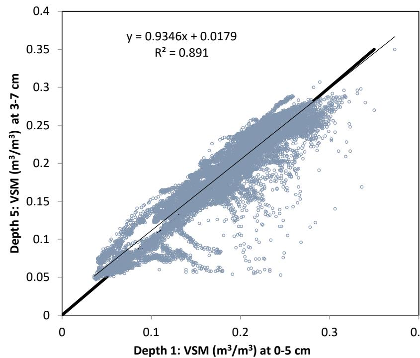
Comparing depths of installation between 2.5 and 5 cm below the surface. Increasing depth yields increased error, on par with error of the instrument of  $0.01 \text{ m}^3/\text{m}^3$ .
