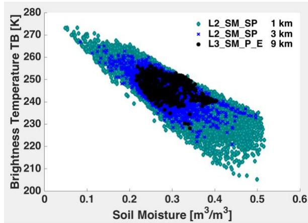
**Figure 17:** Distribution of data in the soil moisture and the brightness temperature space for the L2\_SM\_SP product at 1 km and 3 km, and L2\_SM\_P\_E product gridded at 9 km (~33 km effective resolution) over the Southern part of Iowa on 5<sup>th</sup> May, 2018.
