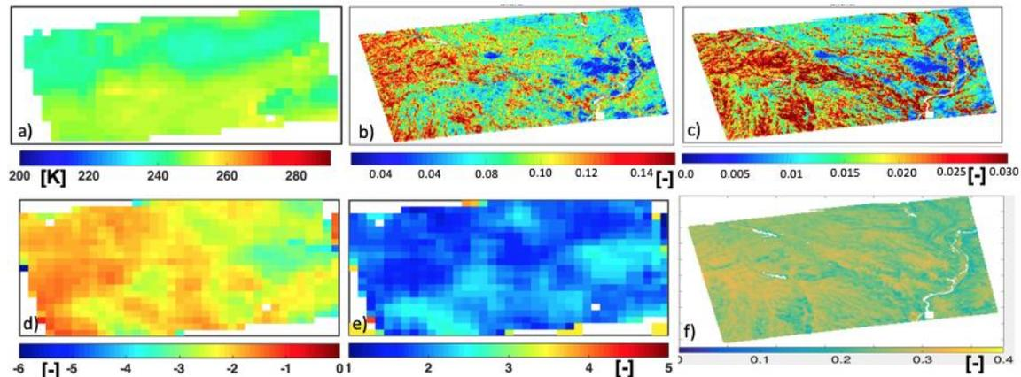
**Figure 15:** An example of primary inputs to the SMAP-Sentinel Active-Passive algorithm. From Southern Iowa, 5<sup>th</sup> May, 2018: a) SMAP radiometer brightness temperature  $T_{B_v}(C)$  at about 33 km resolution but gridded at 9 km; b) Sentinel-1A/B co-polarized backscatter ( $\sigma_{vv}$ ) at 1 km; c) Sentinel-1A/B cross-polarized backscatter ( $\sigma_{vh}$ ) at 1 km; d) Parameter  $\beta'(C)$ ; e) Parameter  $\Gamma$ , and; f) Clay fraction.
