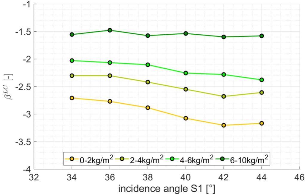
**Figure 6.** Time-averaged (04/2015-04/2017)  $\beta'(C)$  [-] along Sentinel-1A/B incidence angle [°] for four VWC ranges in Africa; circles indicate median values for each VWC range, sourced from [26].
