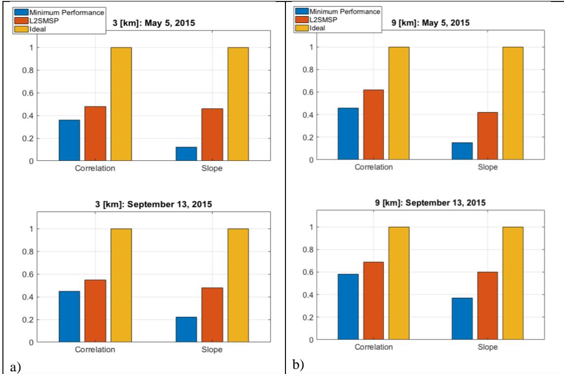
**Figure 13:** a) Bar plots of SMAPEX PLMR observations against L2\_SM\_SP  $T_{Bp}$  at 3 km and Minimum Performance ( $T_{Bv}$  from L2\_SM\_P\_E) at 3 km. b) Bar plots of SMAPEX PLMR observations against L2\_SM\_SP  $T_{Bp}$  gridded at 9 km and Minimum Performance ( $T_{Bv}$  from L2\_SM\_P\_E) gridded at 9 km.
