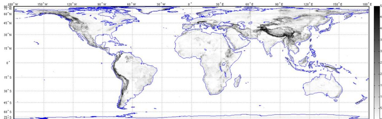
**Figure 25:** Standard deviation in DEM gridded at 3 km EASE2 grid projection.
