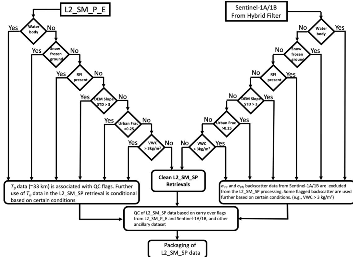
**Figure 26:** Decision Tree to QC  $\sigma_{vv}$  and  $\sigma_{vh}$  from Sentinel-1A/1B and  $T_{Bv}$  from SMAP.
