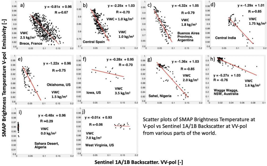
**Figure 3:** Scatter plots between the SMAP L-band radiometer  $T_{B_p}(C)$  and spatially-averaged Sentinel C-band radar data  $\sigma_{pp}(C)$  from various regions of the world.
