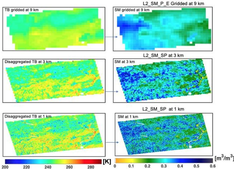
**Figure 16:** Comparison of L2\_SM\_SP product at 1 km and 3 km resolution with the corresponding L2\_SM\_P\_E product gridded at 9 km. The L2\_SM\_SP image is from Southern Iowa, May 5<sup>th</sup>, 2018.
