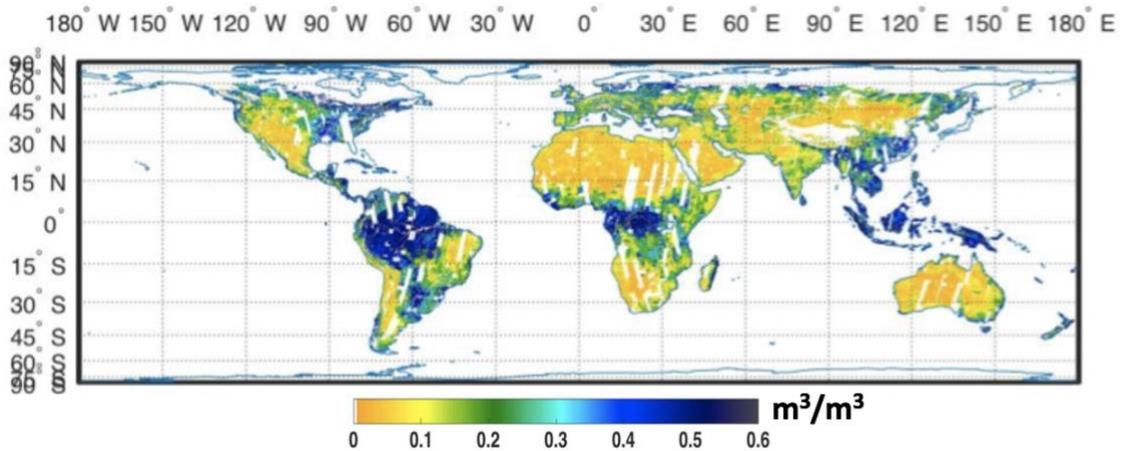
**Figure 14:** Twelve-day coverage of SMAP-Sentinel1 L2\_SM\_SP high-resolution (3 km) soil moisture data from 1<sup>st</sup> May, 2017 to 12<sup>th</sup> May, 2017.
