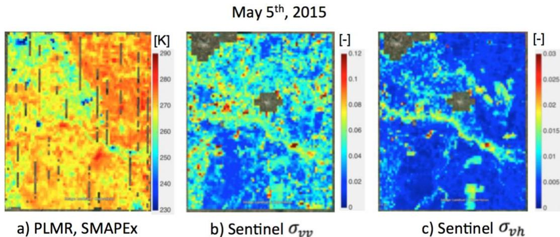
**Figure 11:** PLMR and the Sentinel-1A observations at EASE2 grid 1 km resolution over the SMAPEX study domain on May 5<sup>th</sup>, 2015 (prior to Sentinel filtering).
