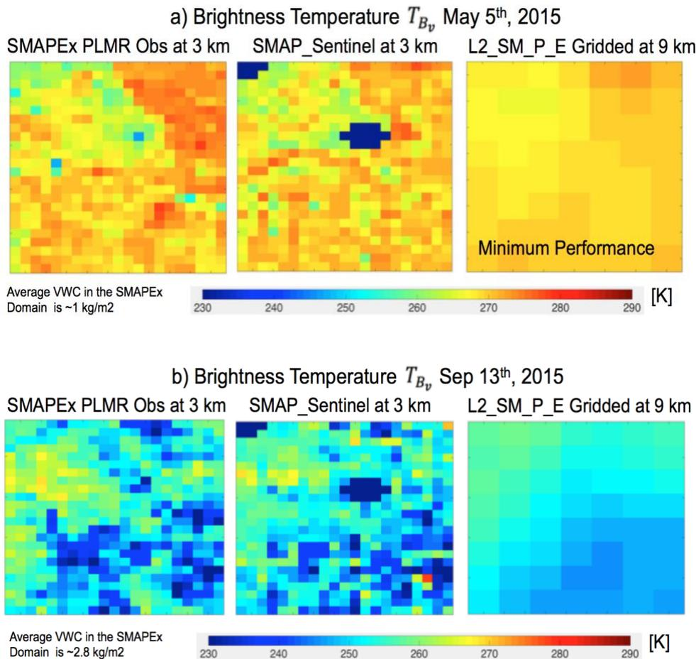
**Figure 12:** Output of L2\_SM\_SP compared against PLMR  $T_{B_v}$  data from SMAPEX and the Minimum Performance ( $T_{B_v}$  from L2\_SM\_P\_E at 9 km).
